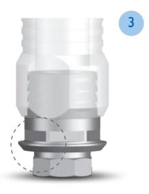
For casting use high-melting cobalt-chrome alloy. Devest gently with ultrasound, water jet, pickling acid or a glass-fiber brush. To remove the oxide layer use glass beads (50  $\mu \text{m}/2{\sim}4$  bar). Be aware of danger of damage of the inner configuration and of the prefabricated connection to implant. Protect carefully the connection to implant during all manipulations with the abutment.
